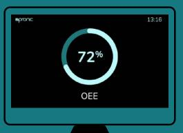
Andon is a method of visual data management, originated in Japan and was developed as part of the Toyota Production System. Andon systems visualize operating states of production lines or individual machines. The information should be displayed in a way that is understandable and immediately recognizable to everyone.
